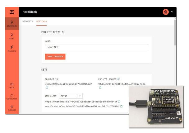
Figure 6. Configuration of our proof of concept in Infura. The Pycom Wipy 3.0 board is also shown.
