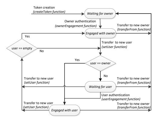
Figure 1. State diagram of smart NFTs.
