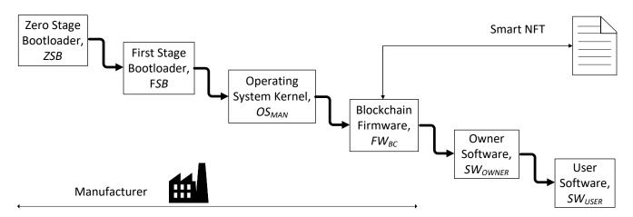
Figure 5. Proposed secure boot process of the IoT device.
