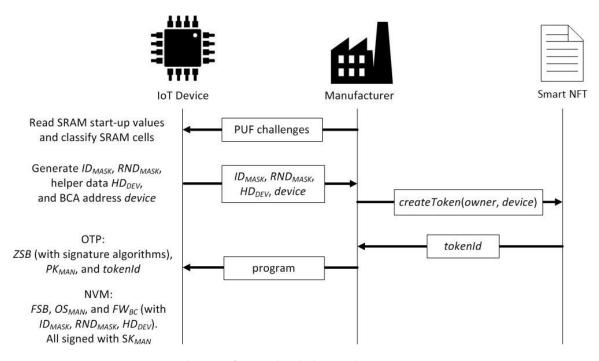
Figure 2. The manufacturer binds the IoT device to its smart NFT.
